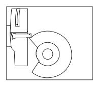
**1.** Remove the outer guard of the grinder. Remove shaft nut and measure shaft size (i.e. 1/2", 12mm, 5/8", 16mm, 3/4", 7/8" or 1").
