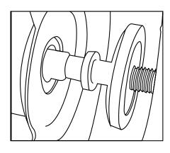
On some machines, there may only be two thin flanges and there may not be sufficient shaft thread to tighten the shaft nut, which may also cause the brush to rub against the inner guard. In this instance, take one of the reducing bushes supplied and use the correct shaft size reducer as a spacer.
