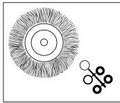
**2.** Each brush is supplied complete with 3 sets of reducing bushes. Match the correct reducing bush with the diameter of your shaft and insert into the 1" hole in the brush on either side. If the brush rubs on the inner guard, refer to the instructions on the next page.
