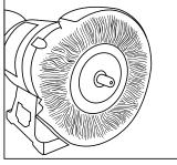
**3.** On most bench grinders there will be a thick and thin flange. The thick flange is generally fitted to the machine side of the grinder and the thin flange to the nut side of the shaft.
